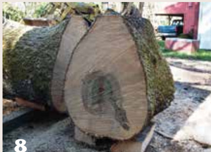
7 As with the straight-grain log, the crotch section is cut apart vertically. Transferring the location of the pith to the top of the log on both ends, as well as drawing the vertical line to the pith, guides the central cut.
