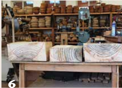
6 With carefully planned and executed chainsaw cuts, the blanks are ready for the bandsaw table, where the bowl blanks are cut round from the square chainsawed blanks. From left: a flat-sawn, natural-edge-oriented blank (but in this case, with the bark eliminated), a quarter-sawn blank, and a flat-sawn blank.
